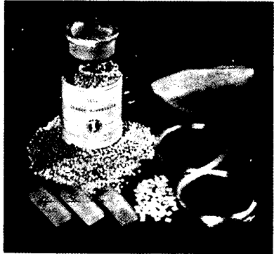
Seed pods of crambe and objects formed from a tough new nylon obtained from erucic acid, the principal constituent of the oil extracted from the seed. Each pod contains one seed. Photograph courtesy of the Northern Regional Research Center, U.S. Department of Agriculture, Peoria, Illinois.
